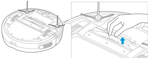
2 Brush roll can be apart by pulling its middle part. Then you can clean threads or hair wrapped around the brush roll by scissors or included brush cleaner.
